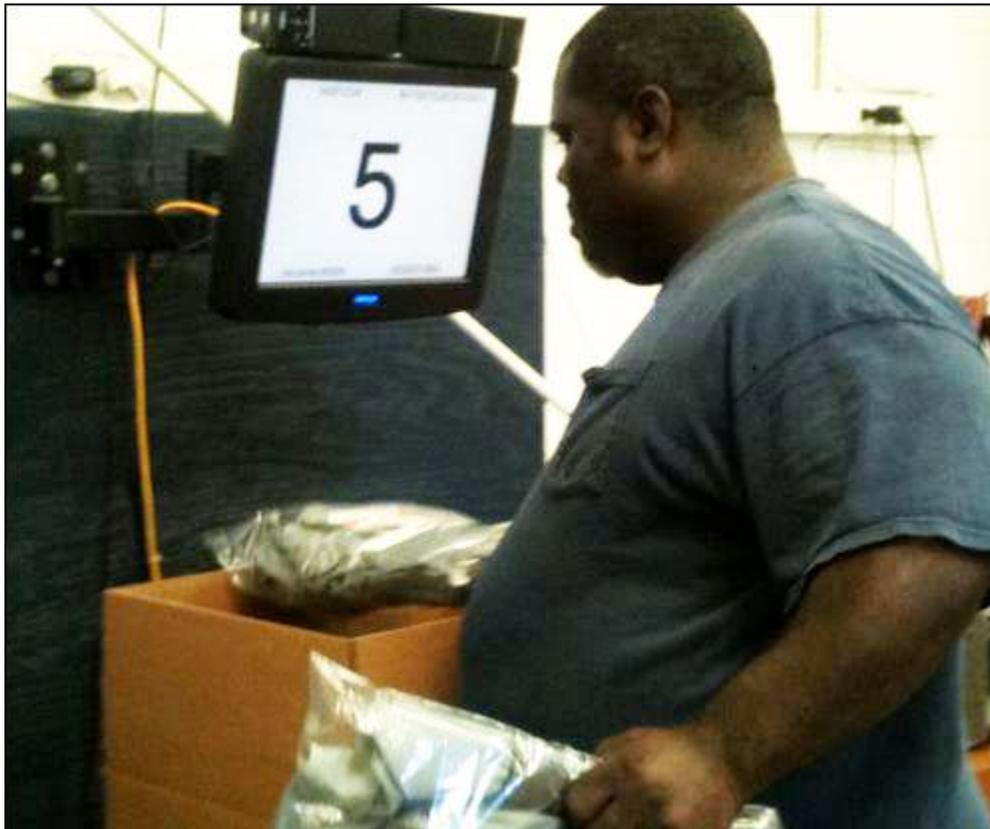
*A ThingMagic Astra reader mounted under a workbench reads the RFID tag of each garment placed in a cardboard box. The system provides a running tally via audio and video.*
