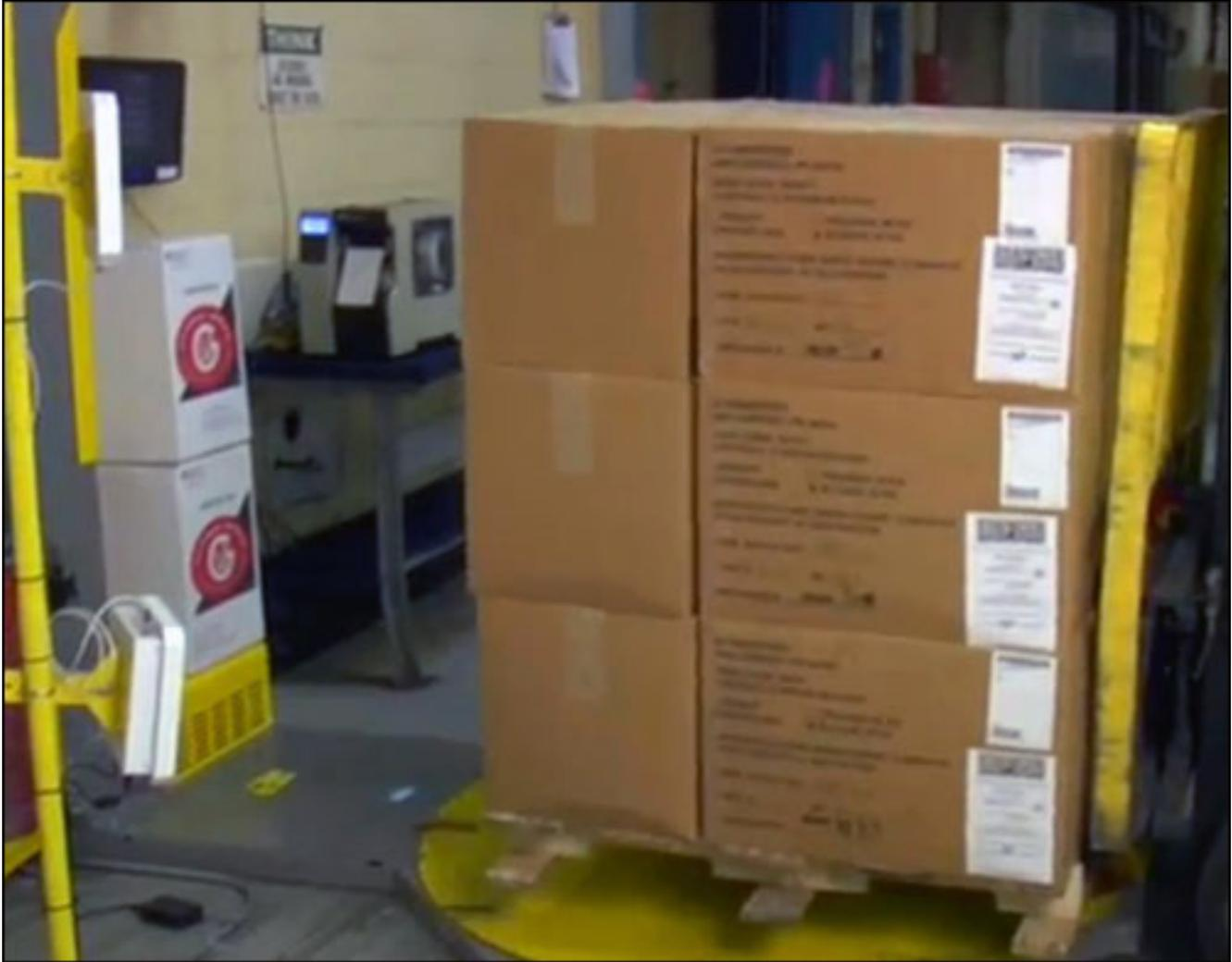
*A pallet loaded with cartons is placed on a stretch-wrap machine, where an RFID reader captures each carton's tag ID number.*
