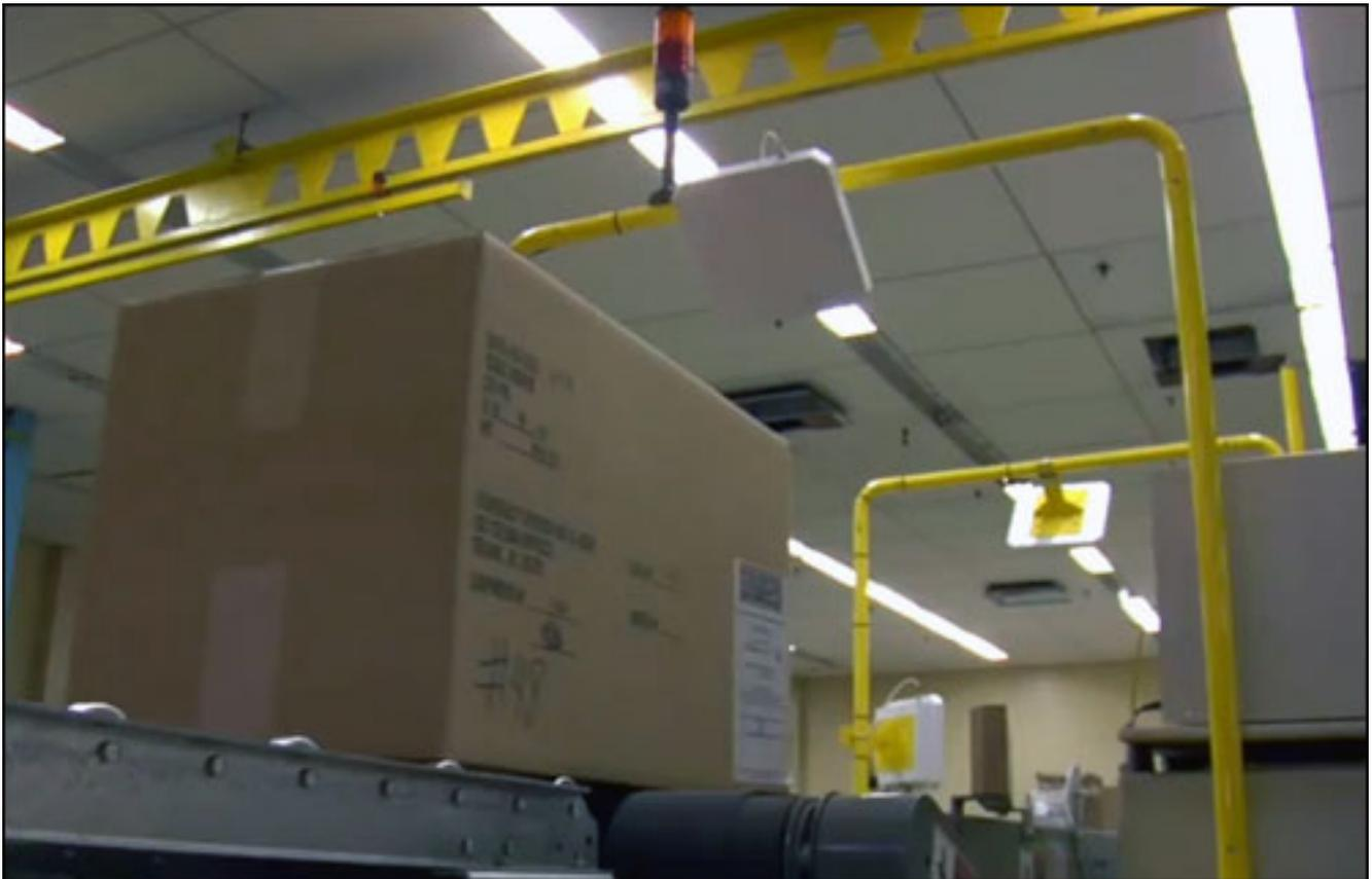
*Cartons filled with RFID-tagged garments are placed on a conveyor, passing through two RFID portals that verify each carton's contents.*
